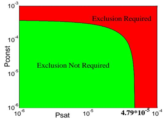
**Fig. 3 Need of Exclusion with Varying  $P_{sat}$ ,  $P_{const}$  for GNSS2 given  $P_{sat} = 10^{-5}$ ,  $P_{const} = 10^{-4}$  for GNSS1**
