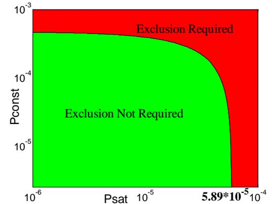
**Fig. 4 Need of Exclusion with Varying  $P_{sat}$ ,  $P_{const}$  for GNSS2 given  $P_{sat} = 10^{-5}$ ,  $P_{const} = 10^{-5}$  for GNSS1**
