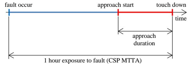
**Fig. A.1 One hour time line for LPV-200 integrity risk requirement interpretation (not to scale)**
