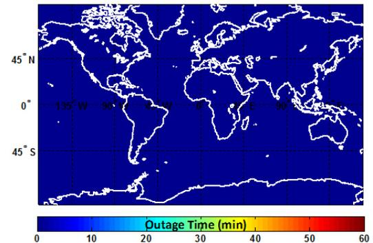
**Fig. 8 Average Continuous Unavailability Duration Using Airborne Detection and Exclusion**
