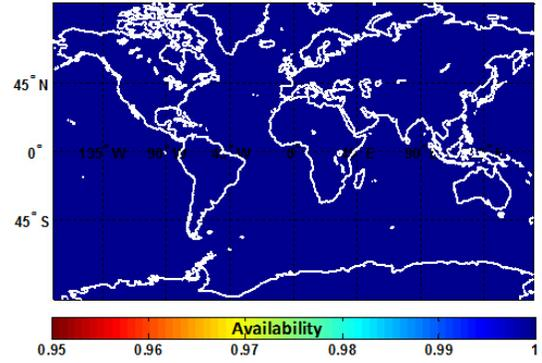
**Fig. 7 Availability of  $P_{HMI} < I_{REQ}$  Using Airborne Exclusion, Coverage of 99.5% Availability is 100%**
