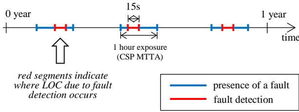
**Fig. 1 One year time line (not to scale), used to interpret the LPV200 average sense continuity risk requirement**
