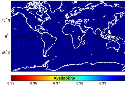
**Fig. 5 Availability of  $P_{HMI} < I_{REQ}$  without Airborne Exclusion, Coverage of 99.5% Availability is 100%**
