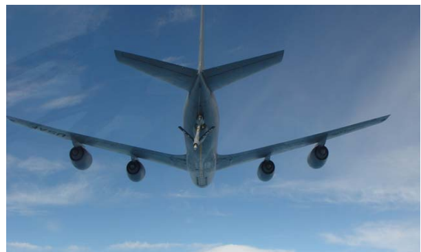
Figure 1: A picture taken at pre-contact position showing the amount of sky blockage introduced by a KC-135 tanker.
