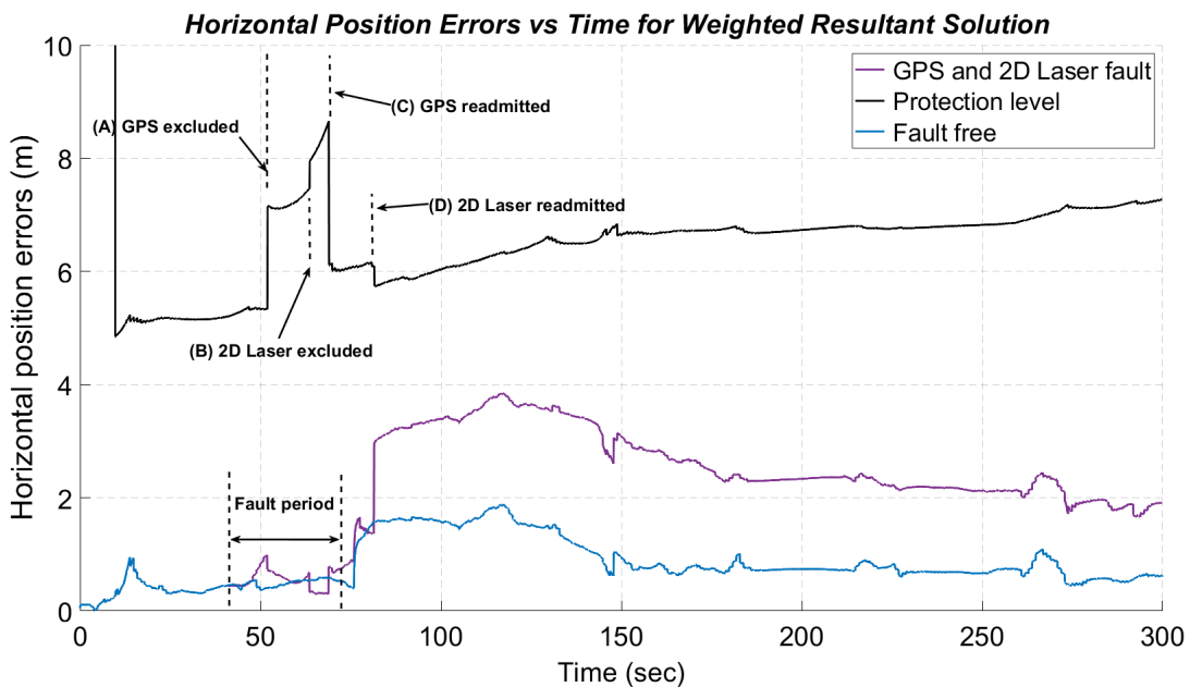
Figure 8: Horizontal Position Errors versus Time for Weighted Resultant Solution (GPS and 2D Laser Fault).
