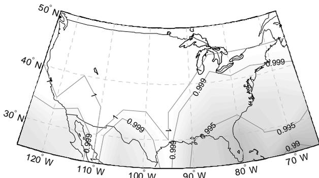
**Figure 7. Availability Map For Dual-Frequency GPS (Single-Frequency Iridium)**
